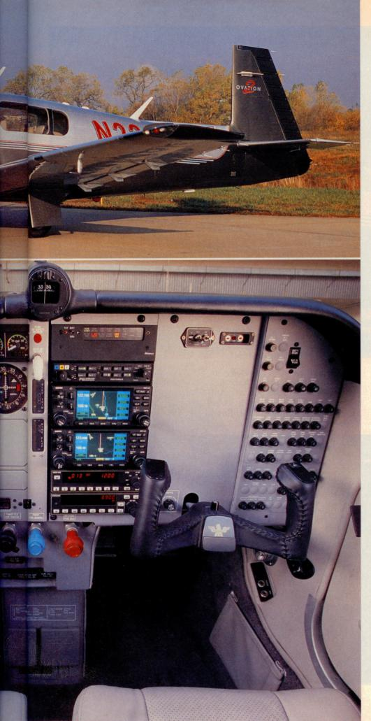
thrust, which hurts takeoff and climb performance. Mooney opted to increase the diameter of the two-blade prop to 76 inches, three inches greater than the Ovation's original three-blade prop. The result is a fair compromise between initial thrust and cruise speed.
