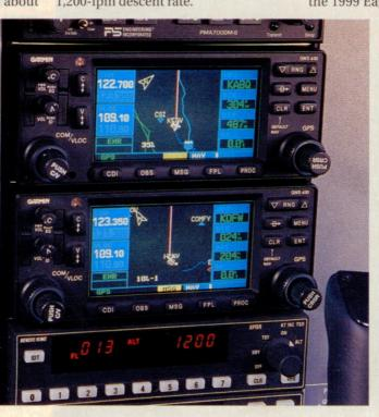
carries dual KX155A nav/coms, a KLN 89B, and the sophisticated KFC225 two-axis autopilot with flight director and altitude/vertical speed preselect. Both models also include an HSI, transponder, and a PS Engineering PMA 7000 audio panel/intercom/clearance recorder.
